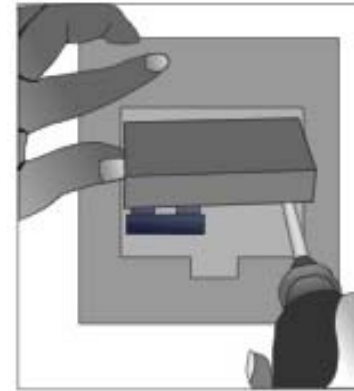
1. Open electrical box
